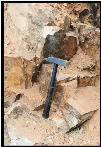
PHOTOGRAPH 7: Three sets of Joint Present at Stone Quarry in Central Range of West Karbi Anglong District.
