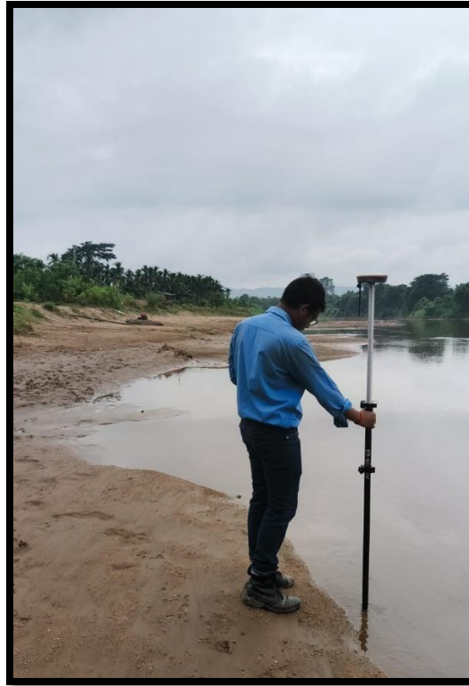
PHOTOGRAPH 4: DGPS survey in Borpani River in West Karbi Anglong District
