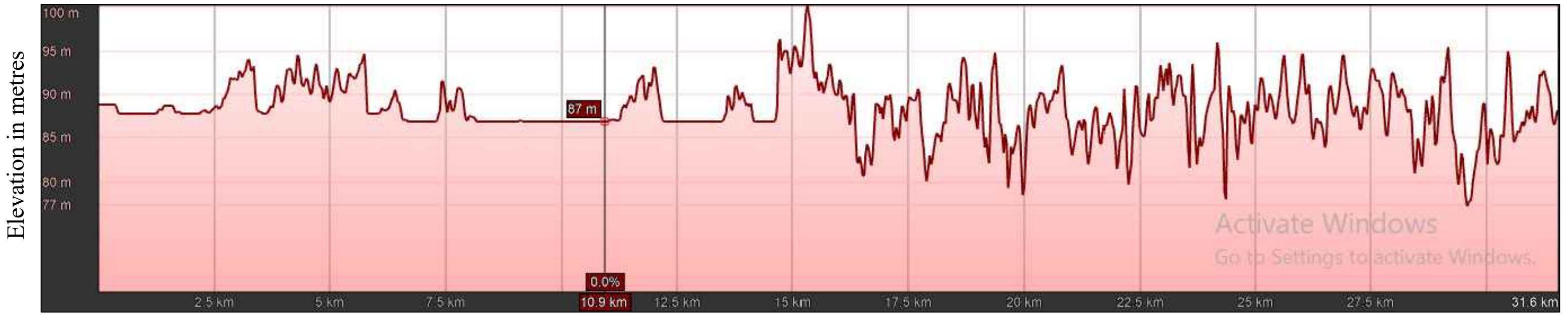
L SECTION OF KOPIL RIVER, KURKUT TO SIBPUR (UP TO 31.6km NORTH TO SOUTH ), (C - C') PART - 03
